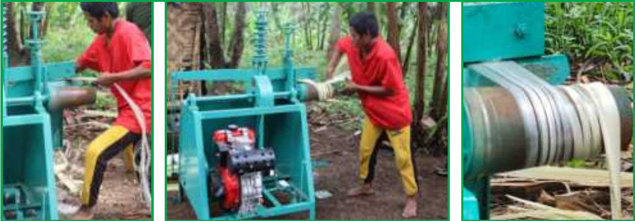
Process of extracting fiber using spindle machine
