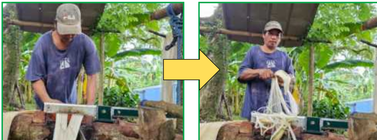
Process of extracting fiber by hand-stripping
