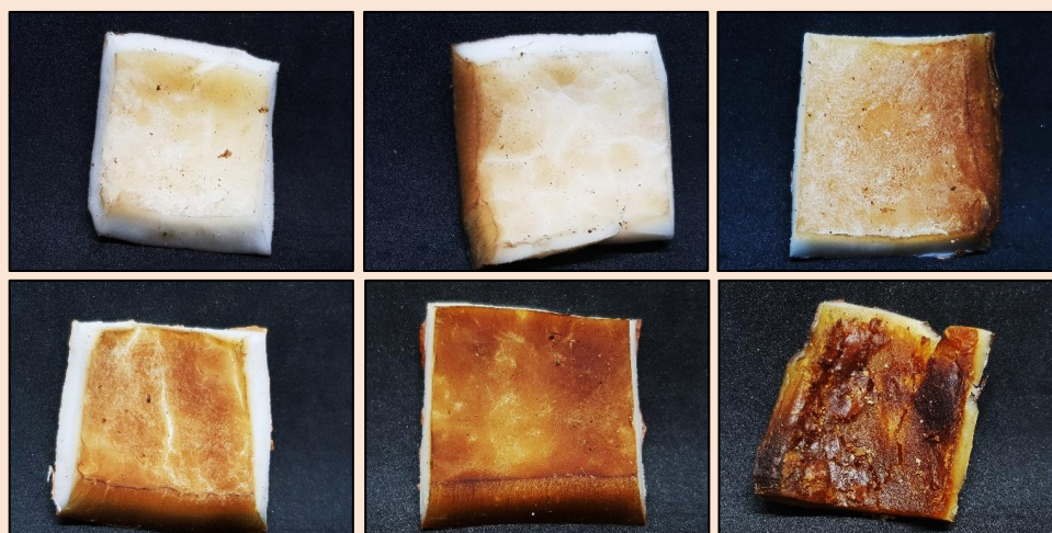
Figure 1. Images of copra from undried to overdried (from upper left to lower right)
