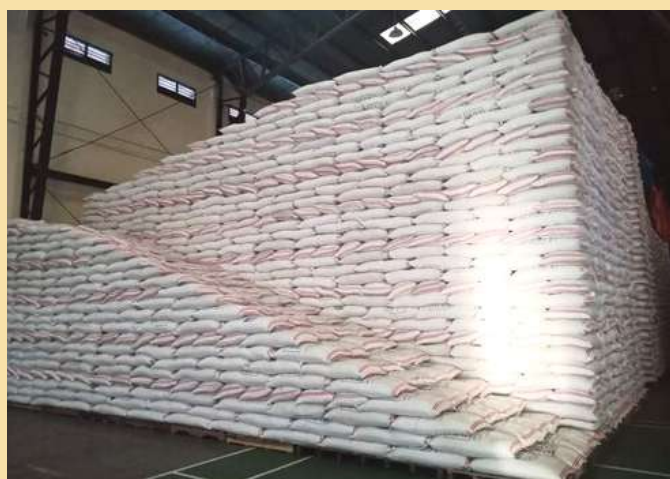
Image 30. Stacked bagged grains in a tight, neat, and squared off manner in NFA warehouse (Source: Gomez, 2021)
