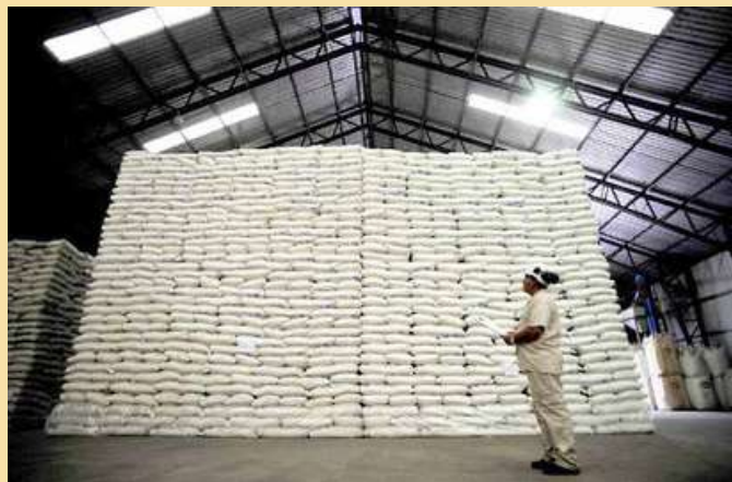
Image 28. Stacked bagged grains in a tight, neat, and squared-off manner (Source: IRRI Rice Knowledge Bank, n.d.)
