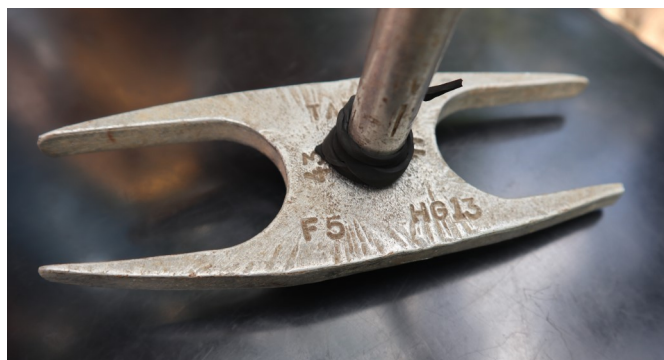
Image 6. Fixed caliper used to determine the diameter of banana finger for calibration
