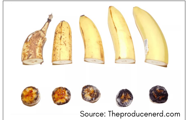
Image 5. Visual demonstration of an iodine test to check the ripeness of bananas
