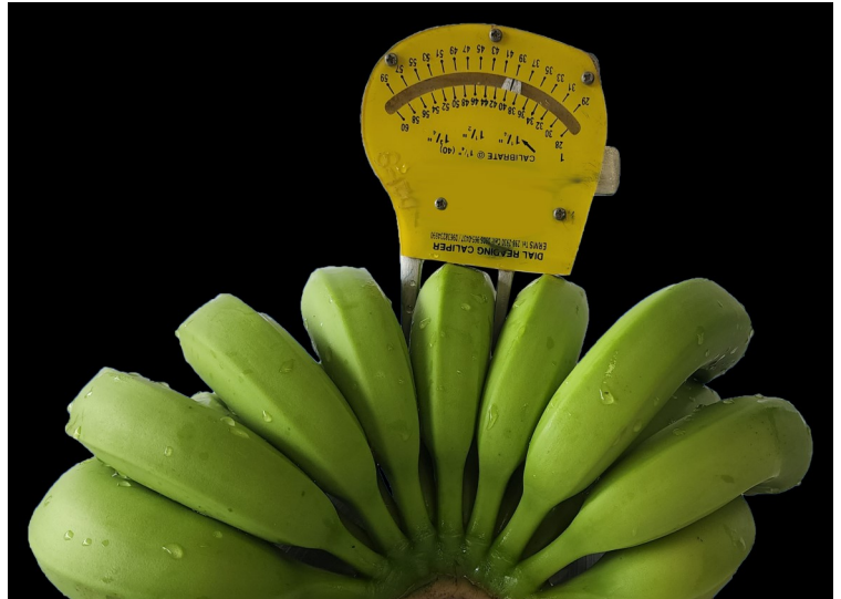
Image 1. Banana diameter measured using a dial reading caliper
