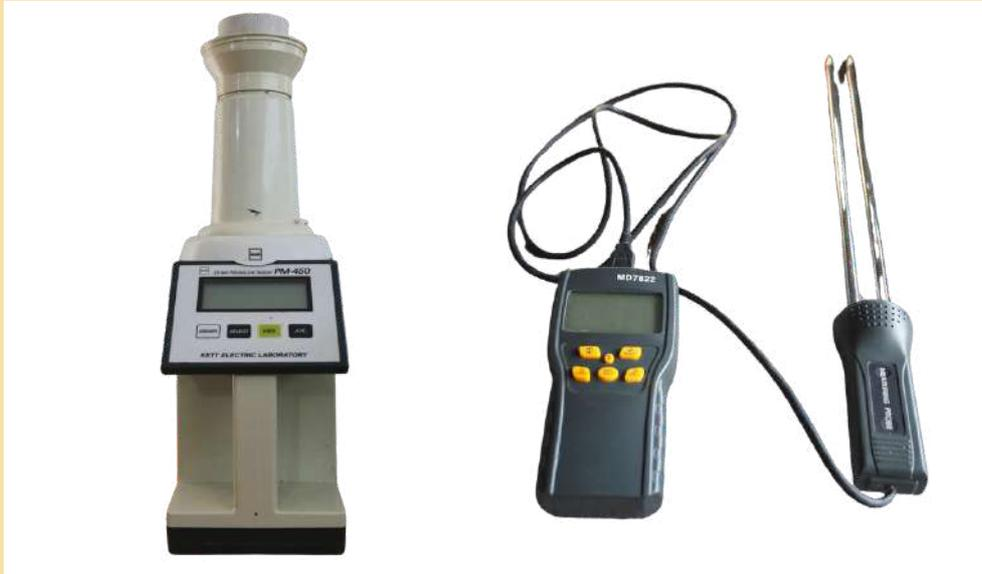
*Image 23. Moisture meters (laboratory or portable) are used for measuring moisture content.*
