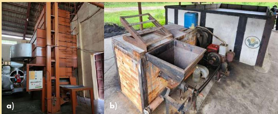
*Image 19. Mechanical dryers used for drying paddy rice - a) recirculating dryer, and b) flatbed dryer*
