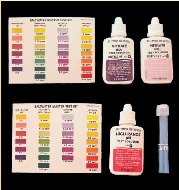
Image 17a. Sample test kit for monitoring water quality in earthen ponds
