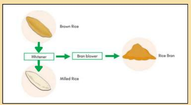
Image 8. An illustration of how dehulled rice is polished
