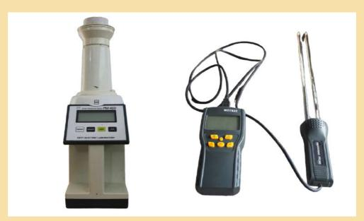
*Image 23.* Moisture meters (laboratory or portable) are used for measuring moisture content.
