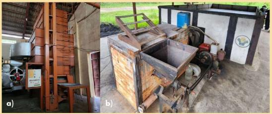
Image 19. Mechanical dryers used for drying paddy rice - a) recirculating dryer, and b) flatbed dryer
