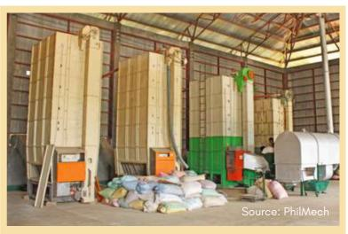
Image 2. Recirculating Dryer can be used for drying paddy rice.
