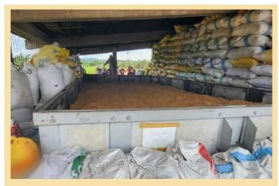
Image 3. Flatbed Dryer can be used for drying.
