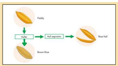
Image 7. An illustration of how paddy rice is dehulled
