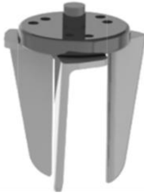
a) rotary tilling blade for vertical shaft type (Azadbakht et al., 2014)
